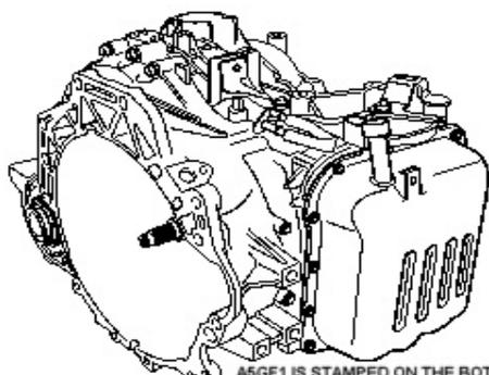
A5GF1 IS STAMPED ON THE BOTTOM OF THE CASE AND CONVERTER HOUSING
