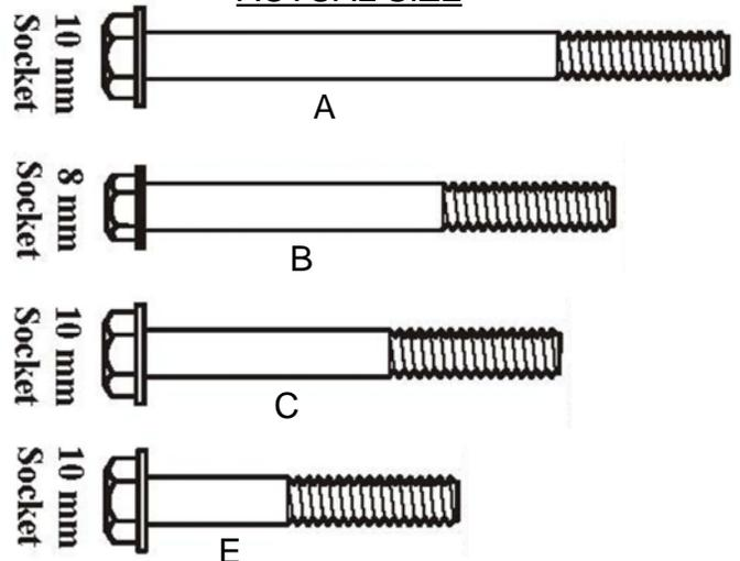
**WARNING !!!** Using an incorrect bolt in this location may lock the gear train and can also damage the case.
